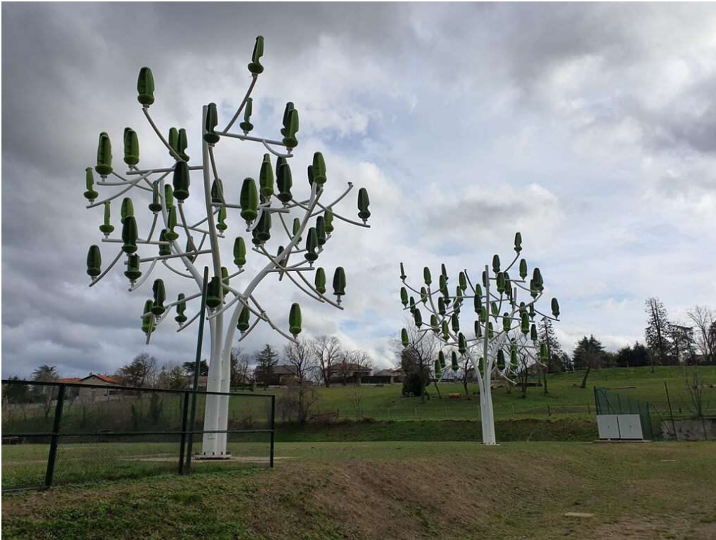
Microwindturbine ism Gebroeders Cappyns.
